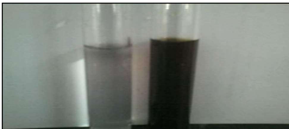
Figure No.1: Aqueous solution of 2mm AgNO 3 before and after the addition of Abutilon indicum L. Leaf broth
